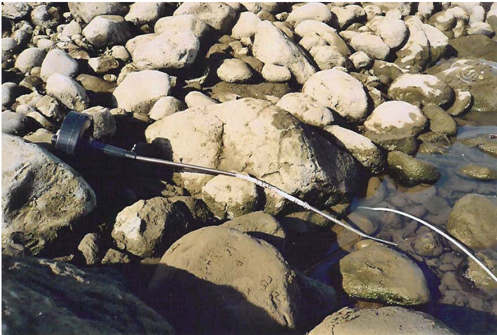
Spring auger (left) after completion of sampling tube installation (right)
