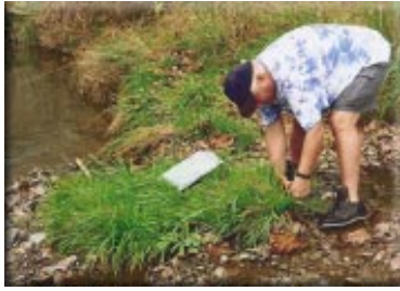
TRAC collected grass from East Fork Poplar Creek to test for artificial radioactivity.
