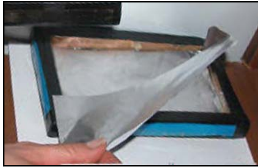
Fig. 2. Placing a number of aluminum foils over the dried sample, before counting [modified from SSGR].
