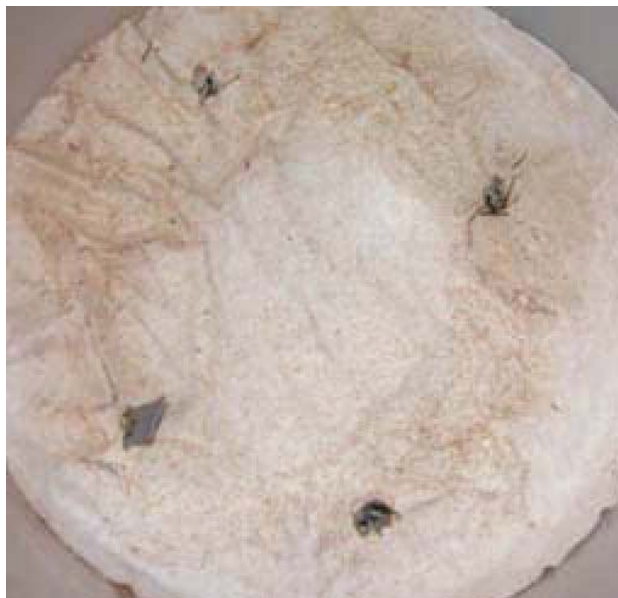
Fig. 4. Coffee filter discolored after filtering creek water for 24-hours [SSGR]. This discolored filter is the original sample for the “Coffee-filtered water sample,” in Fig. 5.
