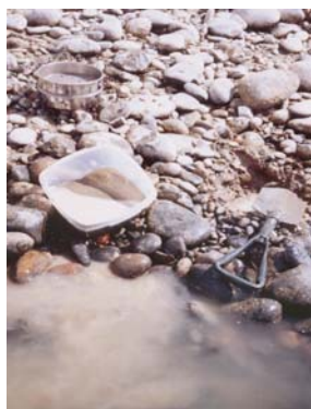
Fig.2.a. Sample in tray, sieve above, and shovel.
