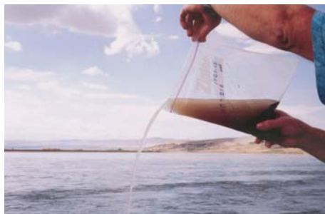
Fig.2.b. Pouring off suspended sediment fraction.
