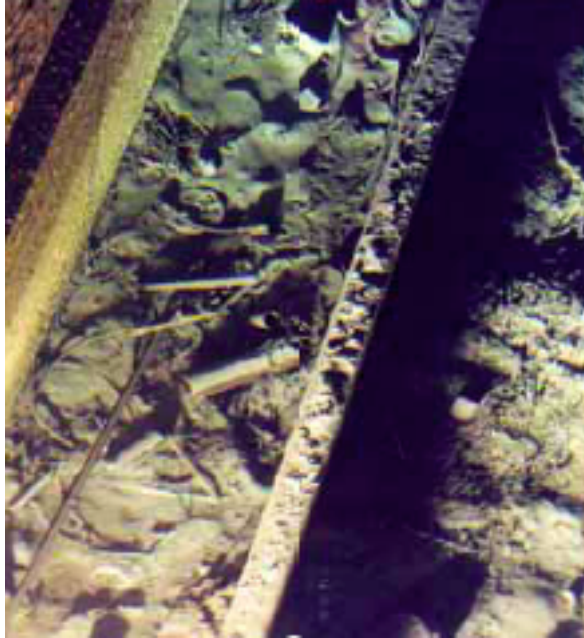
Fig. 4. Sludge in K-East Basin at Hanford [M.W. Peres, "A Comparison of Challenges Associated with Sludge Removal, Treatment and Disposal at Several Spent Fuel Storage Locations, WM'07 Conference, < http://www.wmsym.org/archives/2007/pdfs/7287.pdf > (25 February - 1 March 2007), from Fig. 1].
