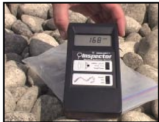
Geiger counter readings on riverbed discharge diffuser head. Background is 60.
